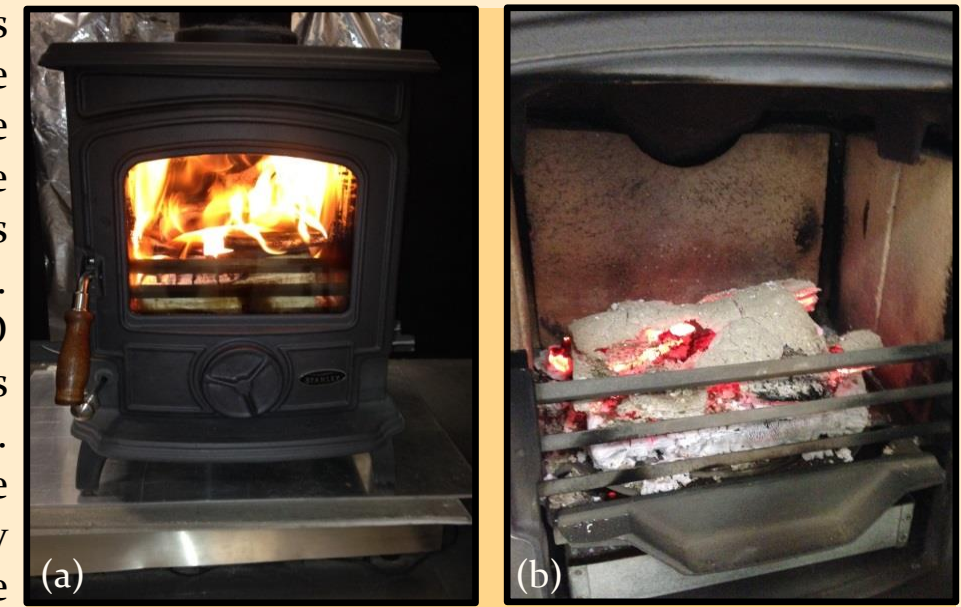
Figure 4: The chipboard/hardwood mix in the (a) volatile and (b) char combustion stages.
