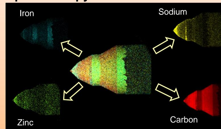
The deposits are mainly carbon based however there are large amounts of sodium and zinc present particularly at the tip of the injector.
