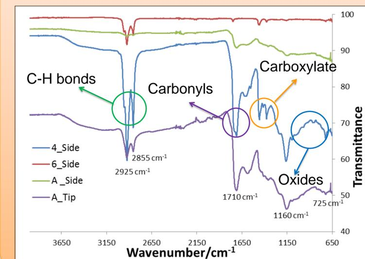
FTIR confirms the presence of sodium carboxylate and zinc oxide salts in the deposit. This indicates deposit formation due to metal contamination in the fuel.
